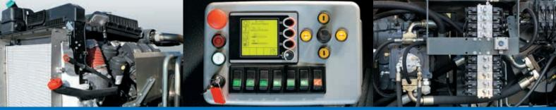
**Powerful engine** The powerful auxiliary engine meeting the latest exhaust emission standards is the heart of our high-performance snow sweepers. **Easy-to-use control panel** Ergonomically and simply arranged, intuitive controls are winning features of this central console. **Central hydraulic system** The central valve block with manual override for controlling the sweeping units is safely housed in the engine compartment.
