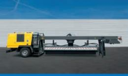
**P 21S as a semi-trailer** This machine boasts working widths of up to 6.3 m for outstanding performance and efficiency, especially at large airports.
